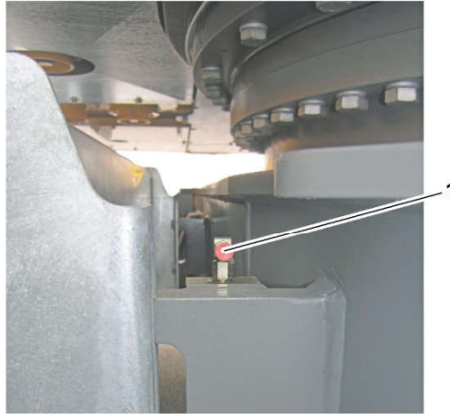
Fig. 739: Oscillating axle central lubricating point
