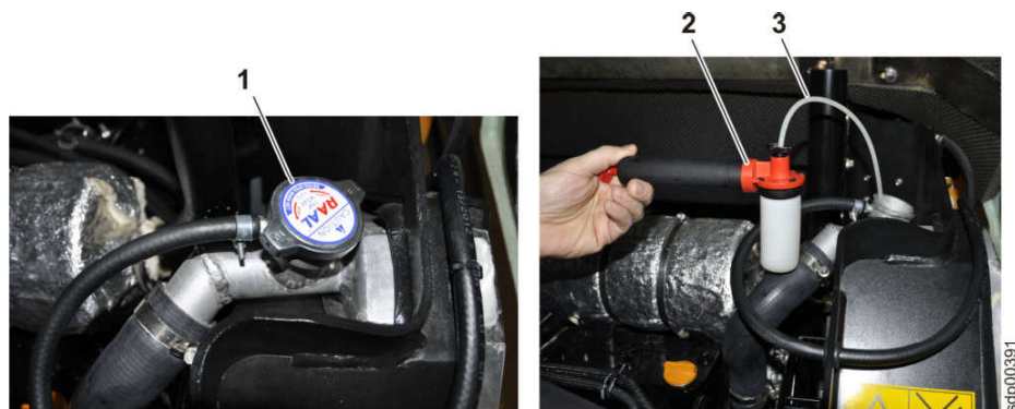
Fig. 203: Sampling point for coolant
