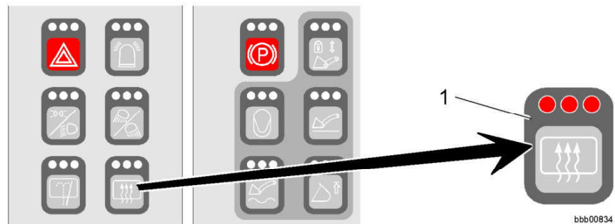
Fig. 257: Switching the rear window heater and mirror heater (optional) on and off
