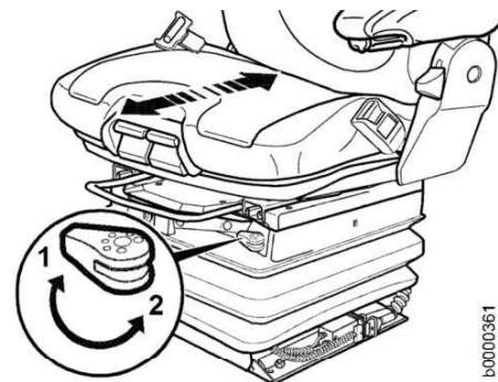
Fig. 105: Activating and deactivating the horizontal suspension on the driver's seat
