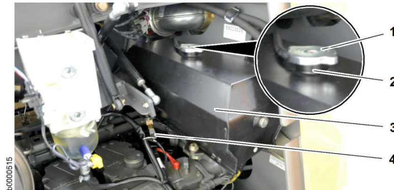
Fig. 306: Checking the antifreeze concentration
