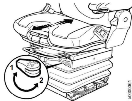
Fig. 106: Activating and deactivating the horizontal suspension on the driver's seat
