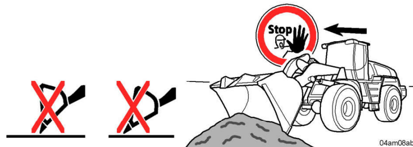
Fig. 384: Impermissible bucket positions
