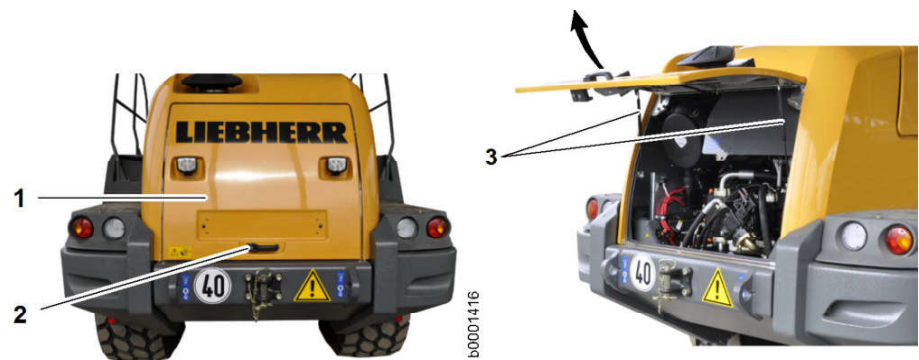
Fig. 280: Engine compartment hatch
