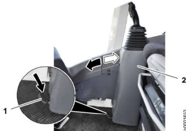
Fig. 85: Adjusting the control panel.
