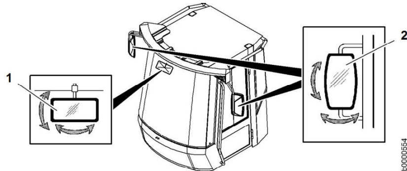
Fig. 98: Adjusting the mirror
