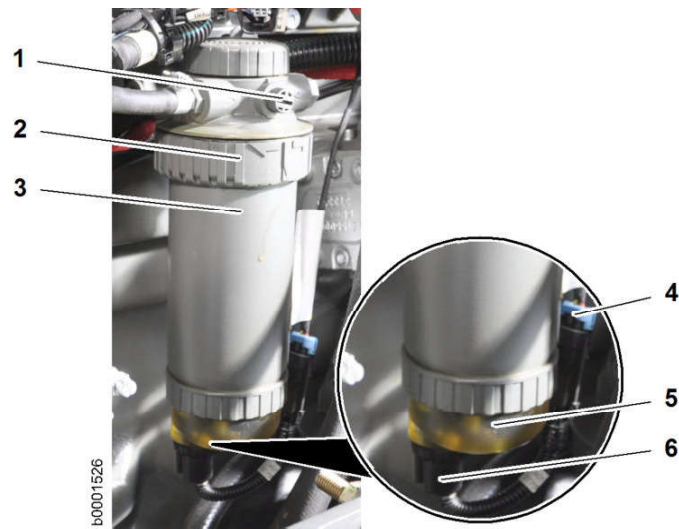
Fig. 224: Changing the fuel pre-filter
