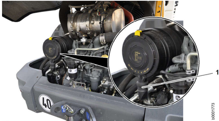
Fig. 304: Cleaning the dust discharge valve
