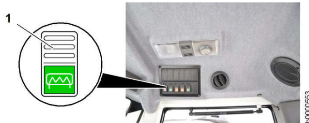
Fig. 158: Switching the rear window heater and mirror heater (optional) on and off
