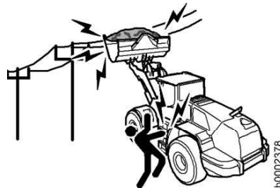
Fig. 232: Working near overhead power lines
