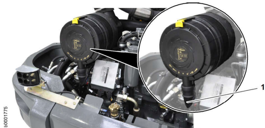
Fig. 246: Cleaning the dust discharge valve
