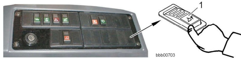
Fig. 242: Switches on the side console
