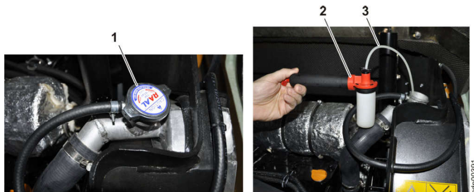
Fig. 198: Sampling point for coolant
