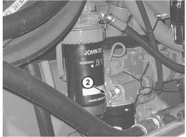
Engine Oil Fluid Sampling Test Port
