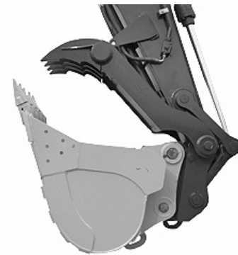
Bucket Rotated to Full-Curl Position
