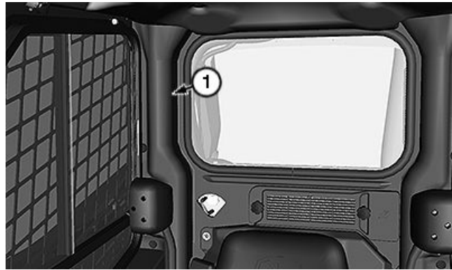
Fire Extinguisher Mounting Location
