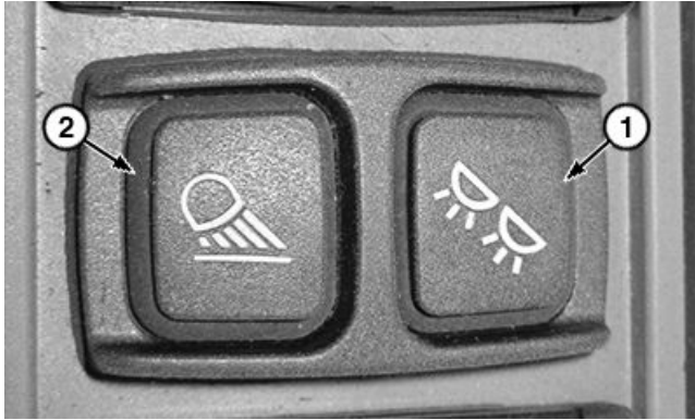
Service and Access Lights Switches (console switches)
