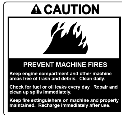
CAUTION, Prevent Machine Fires
