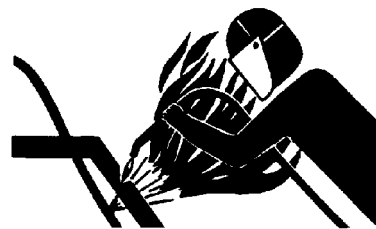
Heating Near Pressurized Fluid Lines
