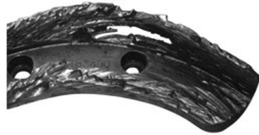
Chain Shot Guard—Perforated
