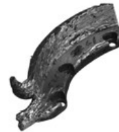
Chain Shot Guard—Peeled and Torn
