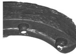
Chain Shot Guard—Worn Thin
