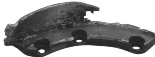
Chain Shot Guard—Edges Worn Away
