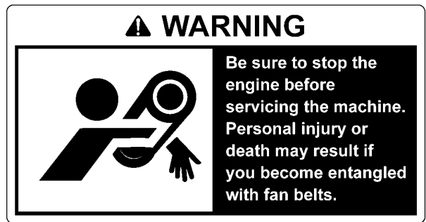
WARNING, Fan Belt
