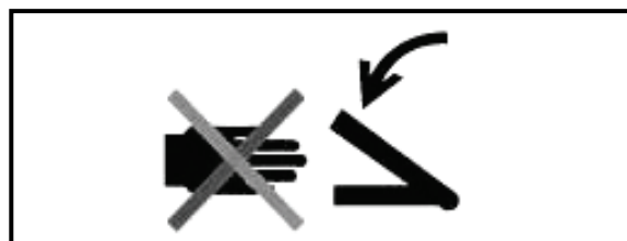
Abb 89. Risk of crushing – do not reach into the area of moving parts
