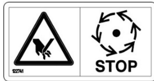
Fig. 9 Overrun time/wait until moving parts are stationary
