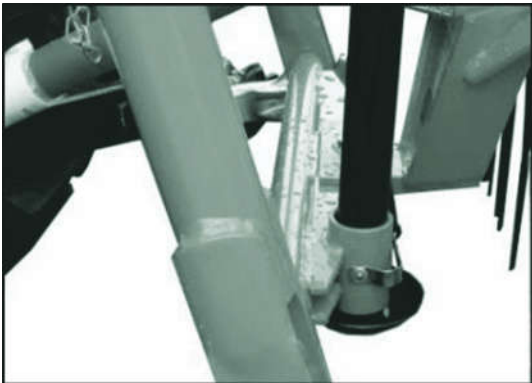
Abb 35. Clip-on bolts on parking support
