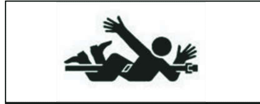
Abb 36. Risk of being caught and tangled on rotating shafts
