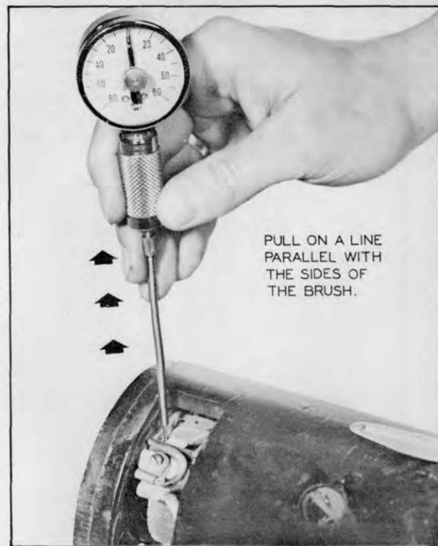
Plate 6450. Checking Brush Spring Tension
