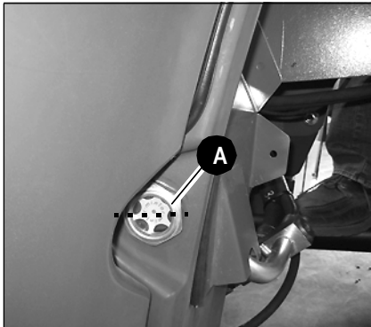
Fig. 179: Oil level sight glass on the hydraulic oil tank
