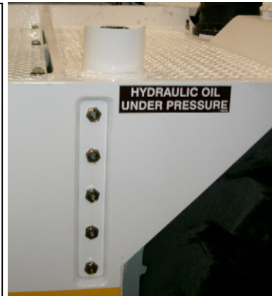
Figure 5.2.1 Hydraulic level sight gauges and filler cap
