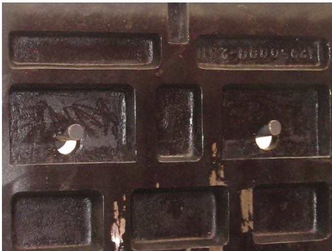
! 3: Make sure the lifting tool is installed correctly in the hole. Lift the fixed jaw plate with a minimum of a 5 ton(Metric) or 6 ton(US) crane.
