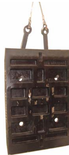
4: Make sure the back of the plate is clean and smooth. Clean out any build up dirt or dust in the holes.
