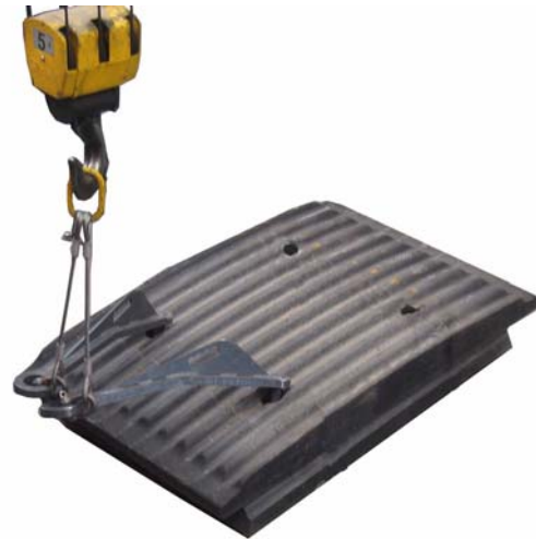
2: Place the lifting tools in the jaw plate. Before lifting the plate make sure the back face and pockets are clean of debris.
