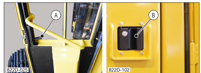
A Side Door Latch (Interior) B Side Door Latch (Exterior)
