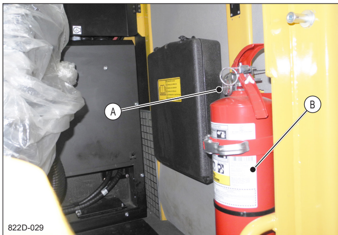
A Pressure Gauge Pointer Must be in Green Zone B Portable Fire Extinguisher
