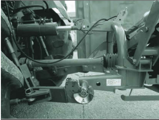
Fig. 21 PTO shaft connections at the same height
