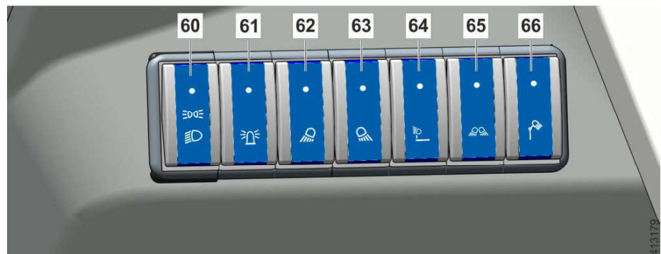
Fig. 125: Control elements - roof console right
