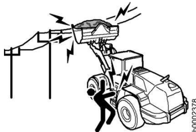
Fig. 276: Working near overhead power lines
