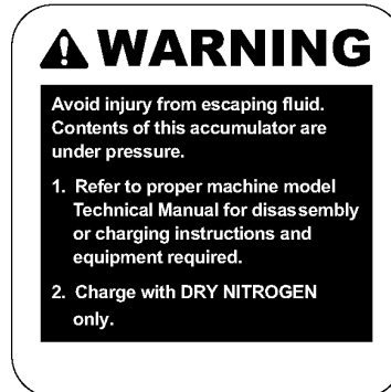
WARNING, Avoid Injury From Escaping Fluid
