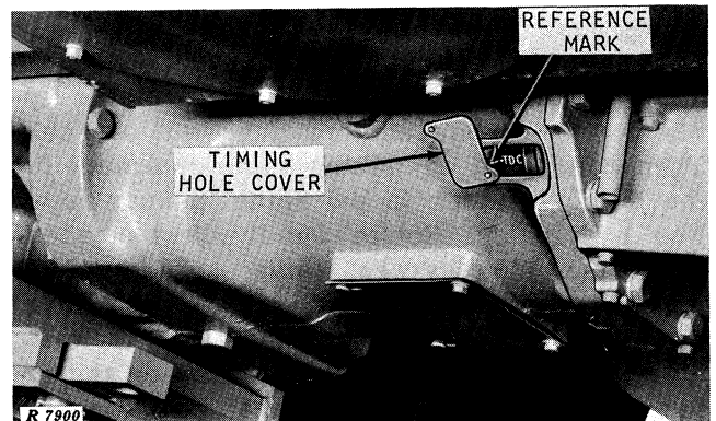
"TDC" Mark on the Flywheel
