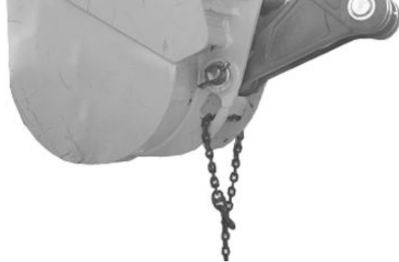
Lifting With Backhoe
