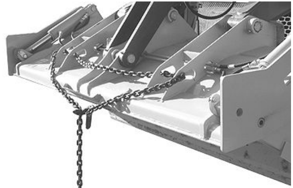
Lifting With Front Loader
