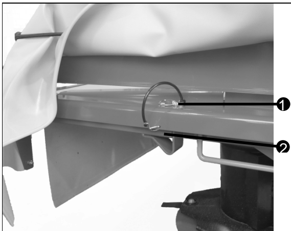
Fig. 39 Support leg lowered
