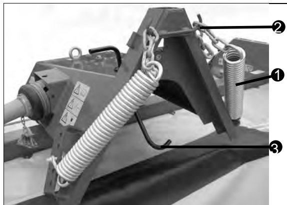
Fig. 40 Storage area for springs and drive shaft holder
