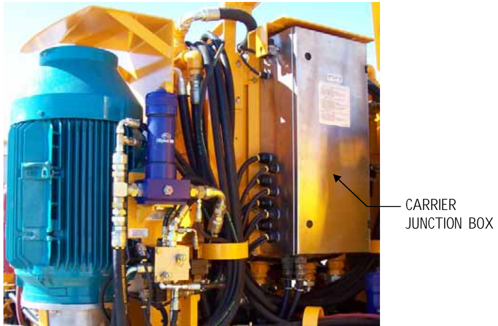
Figure 5 – Carrier Junction Box Location
