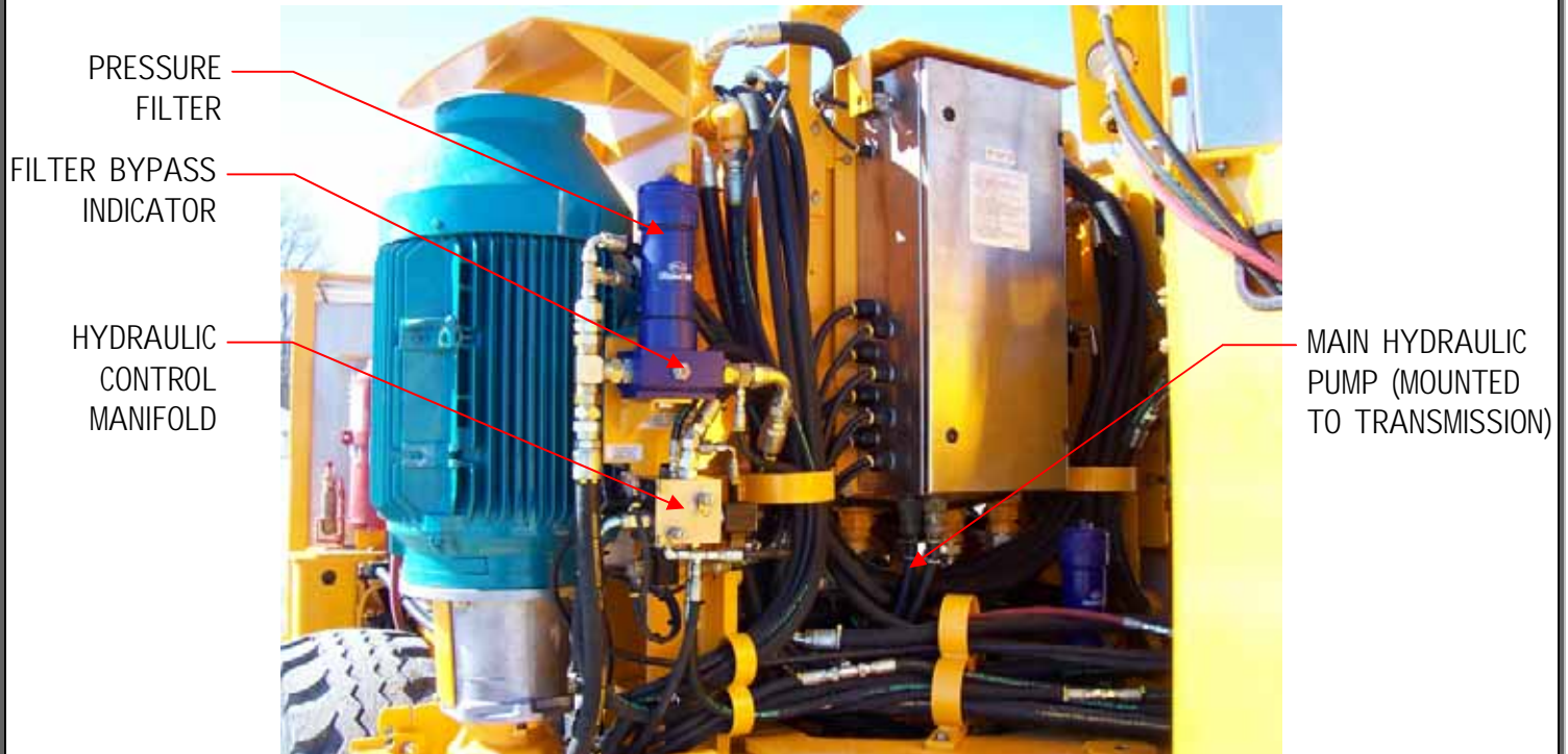
Figure 2 – Carrier Hydraulic Components in Powerframe Assembly Area
