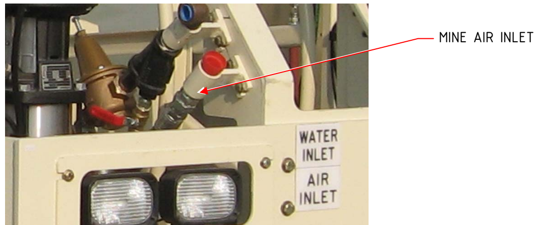
Figure 11 – Typical Mine Air Inlet Located in Rear Deck Assembly
