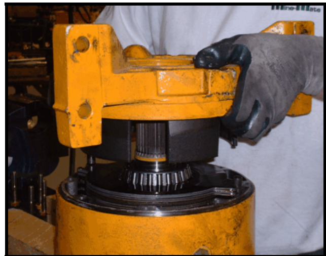
Figure 4- Removal of Power Plate.
