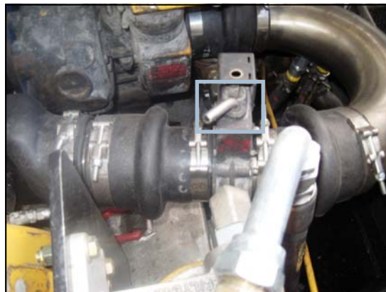
Emergency Intake Shut Off Valve Reset Lever
