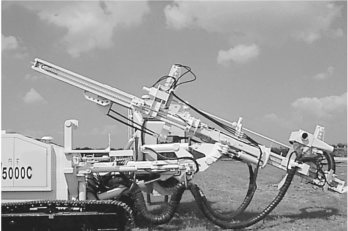
Fig. 4-17 Position of feed and boom when indexing swing cylinder.
