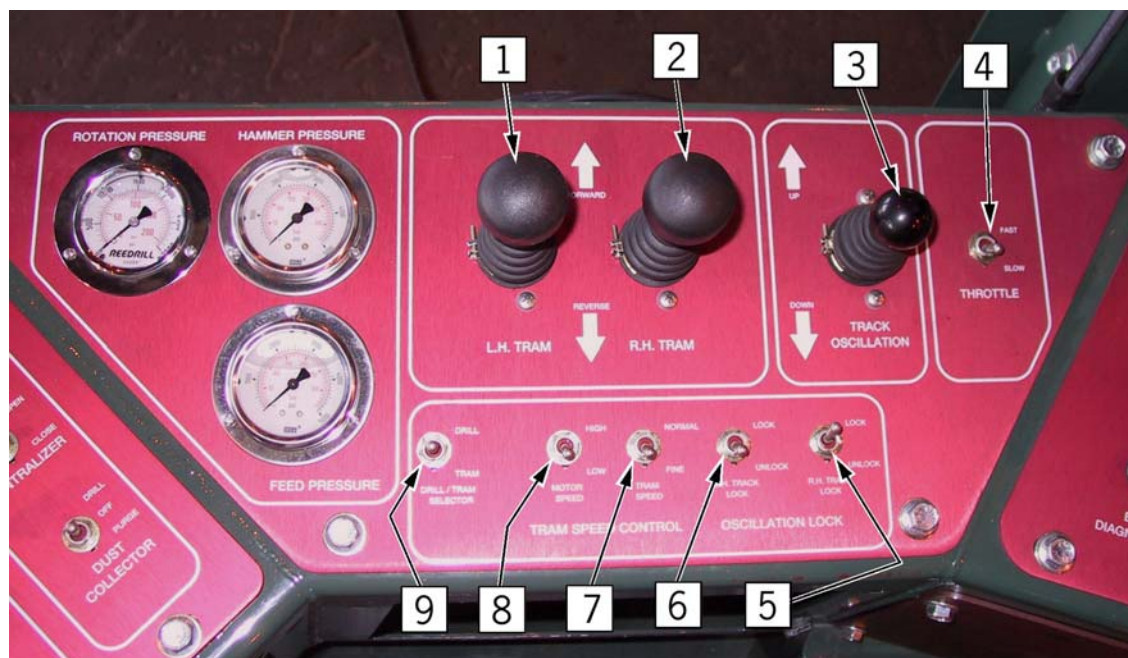
Fig. 3-11 Tram Control Panel in Cab
