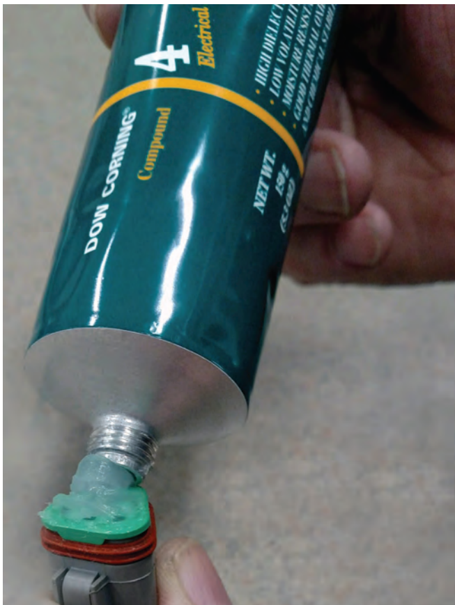
Figure 5-25. Incorrect Application of Dielectric Grease
