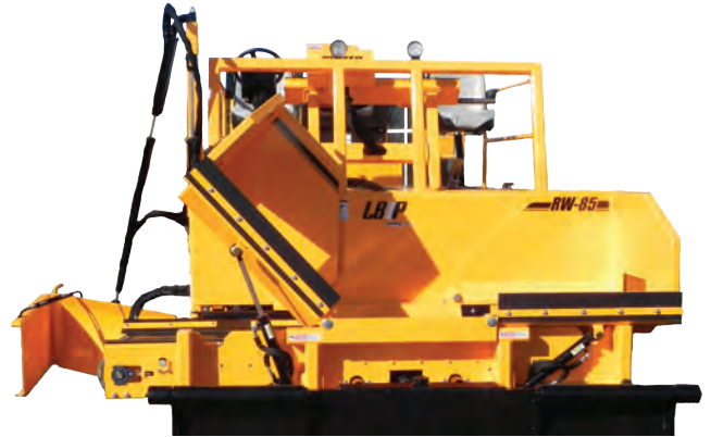
Figure 4-26. Right Hopper Wing Closed with Left Hopper Wing Open
