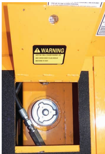
Figure 5-21. Hydraulic Oil Fill Cap
