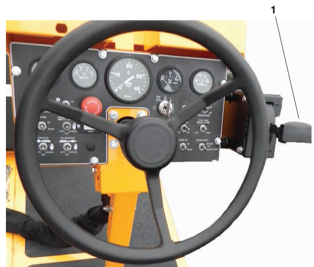
Figure 3-2. Direction-Speed Lever 1 - Direction-Speed Lever Location
