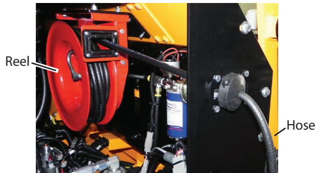
Figure 4-31. Spray Down Hose Reel
