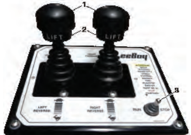
Figure 4-38. Steering and Speed Control Box
