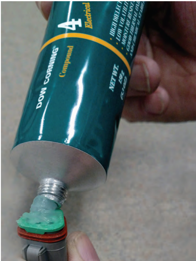
Figure 5-28. Incorrect Application of Dielectric Grease
