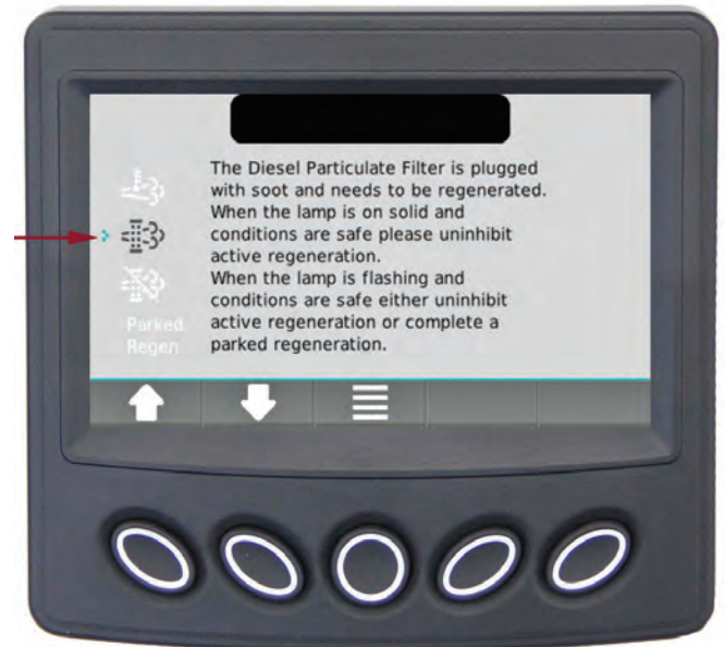
Figure 4-14. Needs Regenerating Screen
