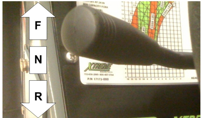
Figure 7-5. Travel Select Lever Must Be In NEUTRAL (N) To Start The Reach Forklift.
