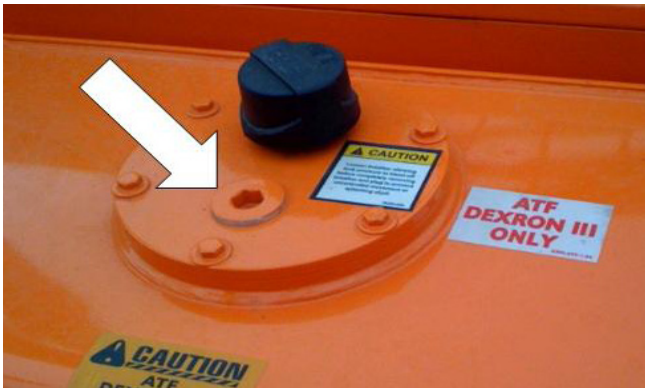
Figure 7-2. Add Hydraulic Oil, If Necessary.
