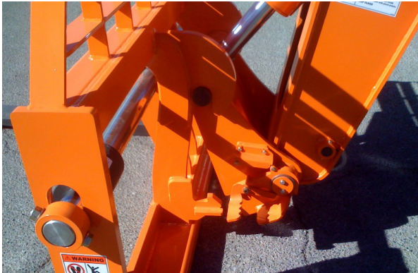
Figure 7-25. Disengage Adapter From Carriage.
