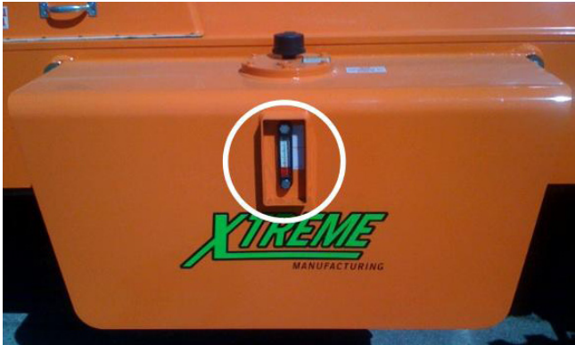
Figure 7-1. Check Hydraulic Oil Sight Gauge.
