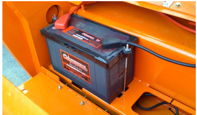
Figure 7-5. Check Battery Case and Terminals.
