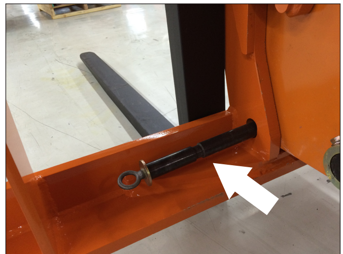
Figure 80. Pull Quick Attach Pin from Attachment and Quick Attach Adapter.
