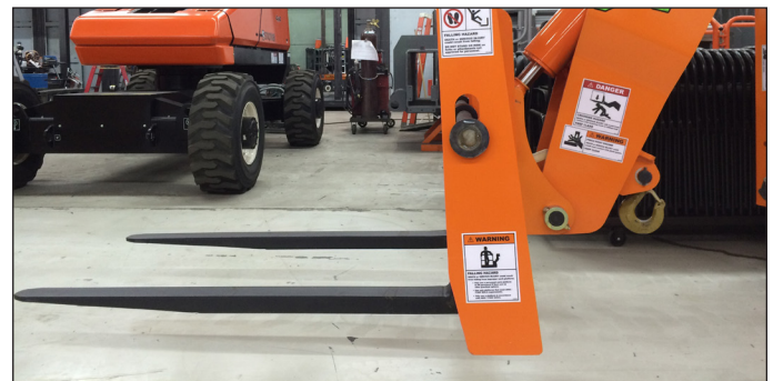
Figure 81. Lower Attachment to Ground in Level Position
