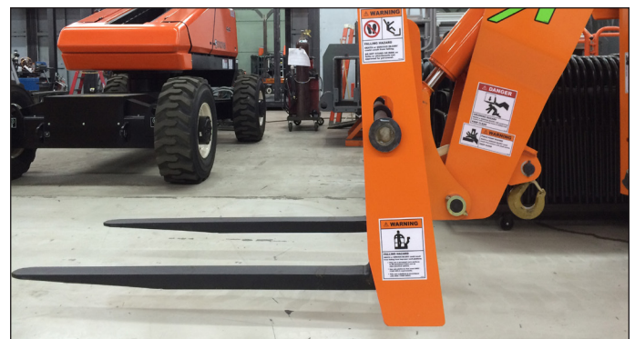
Figure 83. Lower Attachment to Ground in Level Position
