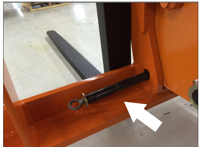
Figure 82. Pull Quick Attach Pin from Attachment and Quick Attach Adapter.
