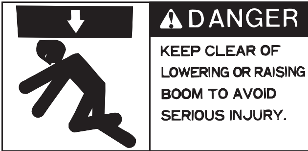
(1) Being crushed by boom
