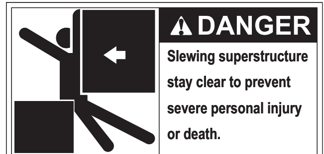
(6) Being crushed by superstructure
